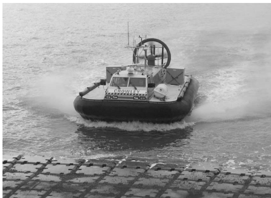
FIG. 2. Griffon 2000TD hovercraft landing on the slope protection mat at Northstar Island's southeastern shore.
