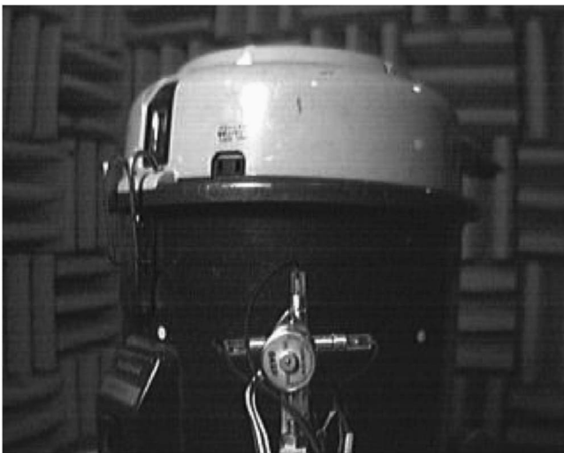
FIG. 13. Picture taken by the CCD camera at the position of the maximum sound intensity of the sound source.
